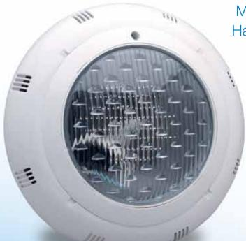
The PROHAYWARD 3640 Nicheless light is fitted with a 100W/12 volt halogen lamp to provide effective pool lighting. Water flows through the rim to help eliminate stagnant water and provide effective cooling for the light housing to assure longer lamp life.
